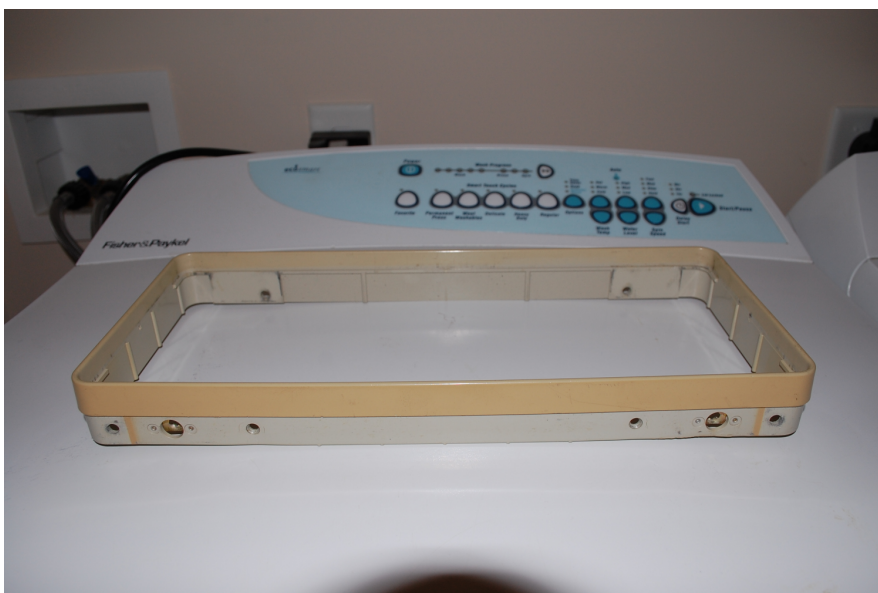
Figure 1: KWM-2 Plastic Trim Ring after 40+ years of discoloration and prior to treatment with the discussed process
