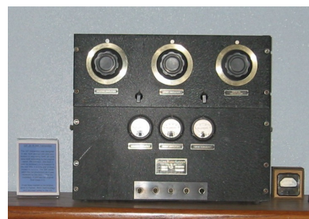
Figure 9: Rare 32F-1 25 watt phone xmtr designed in 1934 and briefly sold in early 1935. Only 25 were made and few remain.
